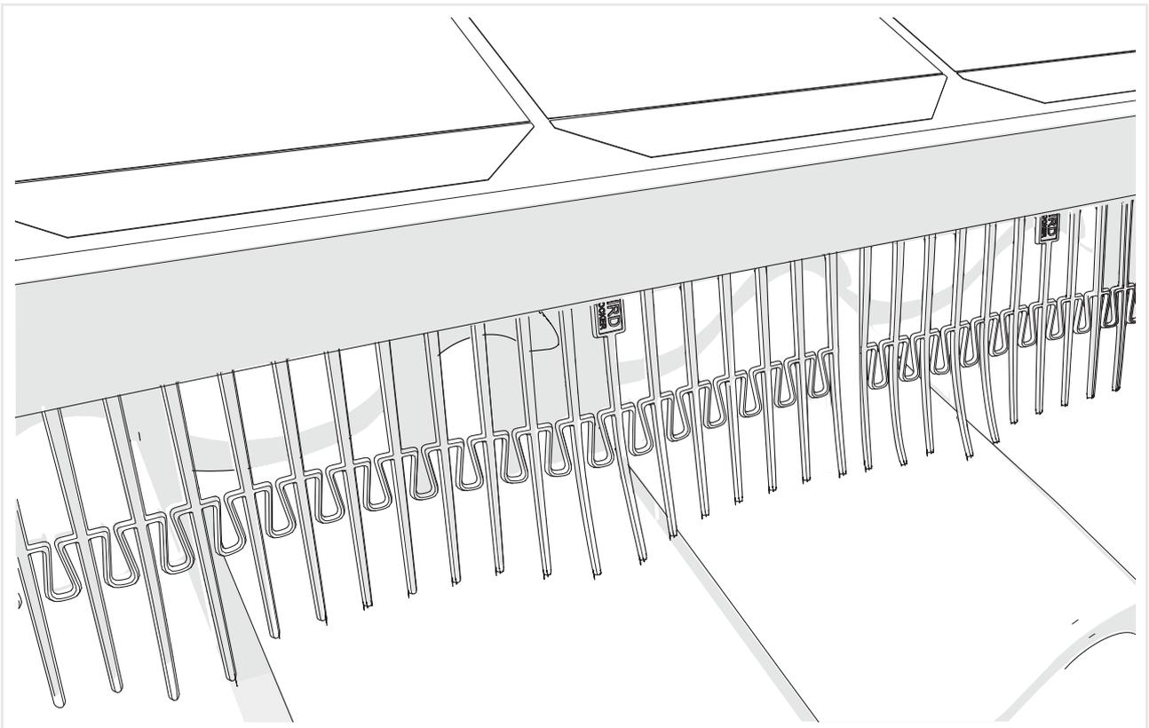
**13** Connect the loose strips together with cable ties.
