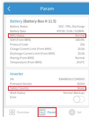
Note: For compatible lithium batteries, the BMS status will display "Normal" after selecting the correct battery company.
