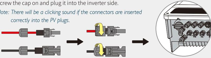
**!** The polarity of the PV strings must not be connected in a reverse manner. Otherwise, the inverter could be damaged.
