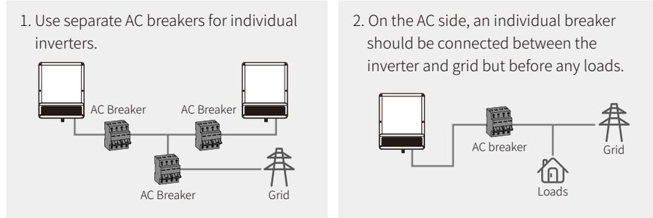
Requirement of AC cable connected to On-Grid and Back-Up side.
