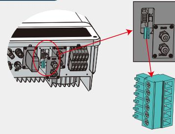
1. Pull out the 6-pin terminal and disconnect the resistor located on this terminal.
